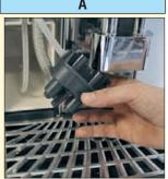
Pull forward the little lever behind the combi spout. Remove combi spout, remove milk hose from milk container and release from combi spout. If a mixer hose is fitted remove it too.
